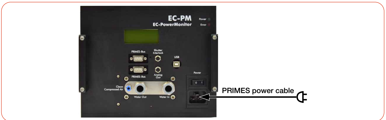
Fig. 7.3: Power supply via PRIMES power cable, display of the measured values on the device
